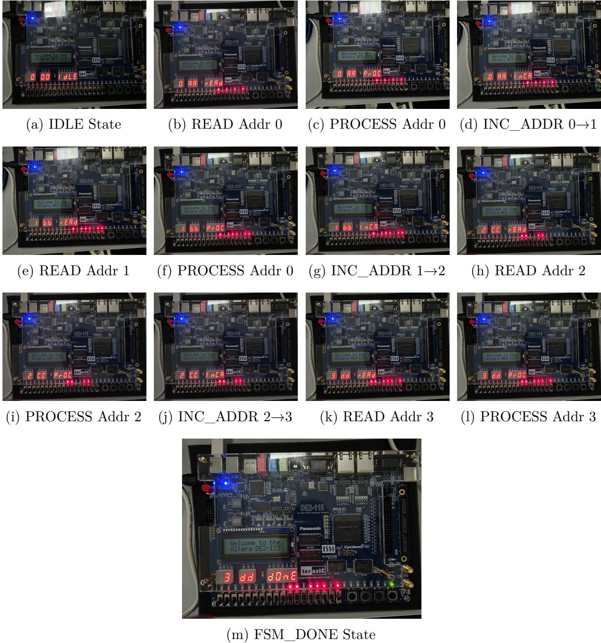
Figure 10: FPGA Implementation of Memory-based FSM - Complete Memory Access Sequence
